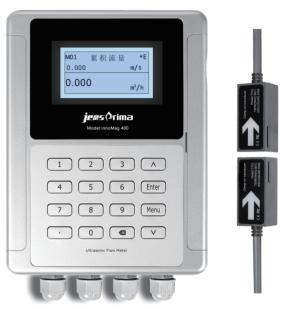
innoMag 400 is an ultrasonic flowmeter based on the principle of time difference time measurement, consisting of a controller and an external clamp-on sensor. Just paste the external sensor on the surface of the pipe to complete a variety of liquid flow measurement, compared with the traditional flowmeter, it does not need to break the flow of the short pipe, easy and fast installation, truly non-destructive installation.
