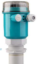
innoLev 300 ultrasonic open channel flow meter using first-of-the-art, non-contact ultrasonic measurement technology, based on the standard installation sink and weir, observe the height of its water level, and thus calculate the flow.
