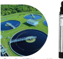
The InnoSens 810T high range turbidity sensor with 90° light scattering technology and conforms to EN ISO 7027. As light passes through the solution, part of it is absorbed and scattered and the other part is transmitted through the solution. This allows the turbidity/suspension of a water sample to be measured by measuring the intensity of the scattered light from particles in the water up to 4000 NTU.
